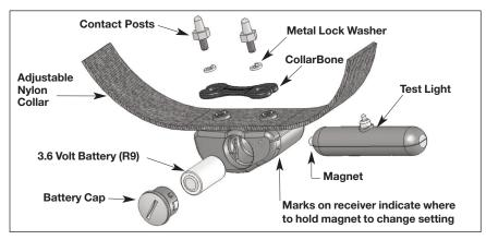
The components of both the R9 (above) and the R7m are the same except the R7m is smaller and uses a different battery.
