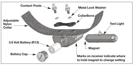
The components of both the R12 (above) and the R12m are the same except the R12m is smaller and uses a different battery.
